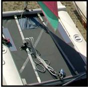
The tighter the toestraps, the less effort it seems to take to hike out. It is also much easier to get back in the boat as your feet aren't as high! The boat on the left has the Velcro tension adjustment at the front. It is almost impossible to get these tight enough and they should be replaced with ones with rope at the front. A good rule of thumb is that the straps should be tight enough so they don't touch the tramp (right) and the tighter the better.
